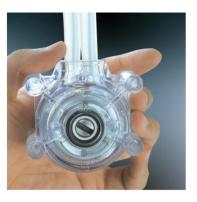
3. Tighten the tubing aptly, and load the other half pump head body.
