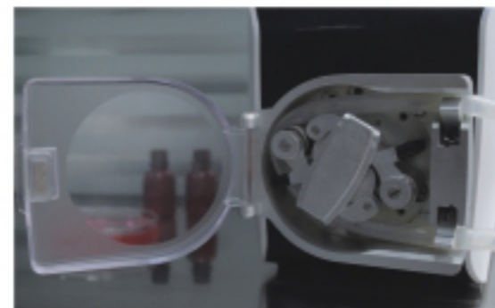
3. Press the pipe clamp, put the tube into the U shaped groove.
